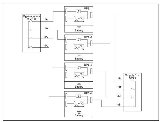
Figure 21 Bypass wiring diagram and cable length notes
